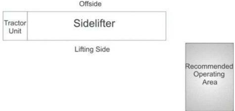
This is a view from above. Operator stands on the lifting side at least 2metres back from the rear of the Sidelifter where he has a clear field of vision of both the lifting side and rear of Sidelifter. This position is also recommended for transfer to or from a companion vehicle
