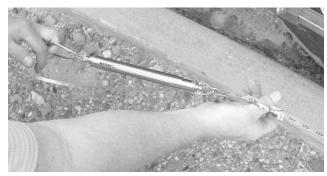
Figure 18. Using the tape tensioning device
