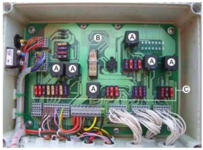
This is the main junction box where most fuses and relays are found. Controls engine functions.
