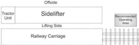
For transfer to or from a railway carriage, the recommended Operating Area is at least 2m back from the rear of the Sidelifter, close enough to the gap between the Sidelifter and carriage to be able to see both.
