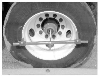
Figure 16. Installed wheel-end extender
